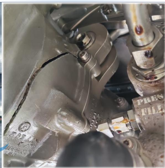
Figure 1 || Engine no.1 and crack found in EGB casing
