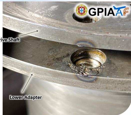
Figure 7 || Heat spots detected on the ADS assembly and lower coupling
